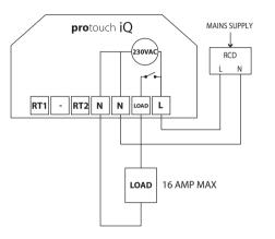
This product must only be installed by a qualified electrician and comply with local installation regulations.
