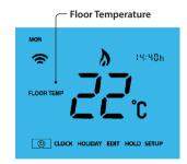
When the ProTouch iQ is set to use both the air & the floor sensor, the room temperature will be displayed by default.
