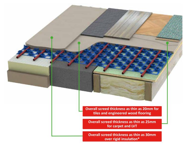
\*150 kPa compressive strength @ 10% compression (minimum) and taped joints
