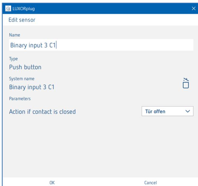
The setting "Operation with closed contact" depends on the contact used (NO contact (NO) or opening contact (NC)).
