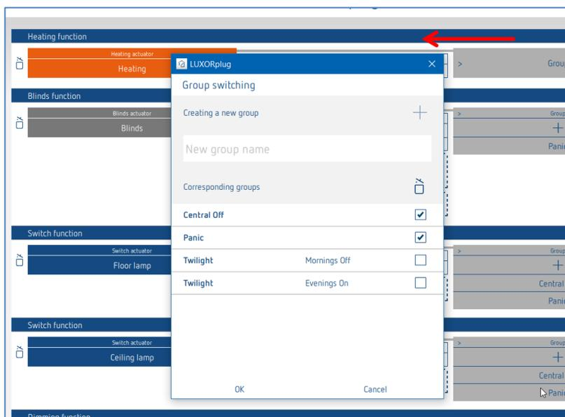
Here, the channel can be integrated into existing group functions, and own groups can be added. The thresholds for twilight functions can be set in the settings of the weather station.
