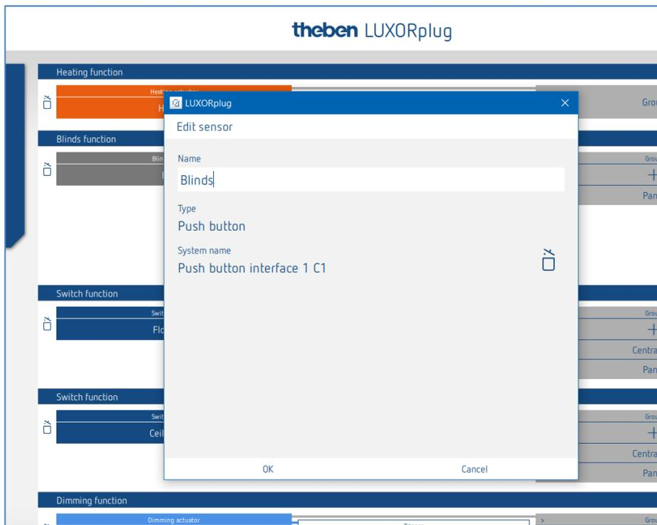
For controlling blinds, roller blinds, or an awning, two inputs are necessary (Up/Down). This input pair will be assigned automatically. The first trigger that is assigned must have an odd channel number (C1, C3, C5, C7), and the second trigger will be added automatically (C2, C4, C6, C8).
