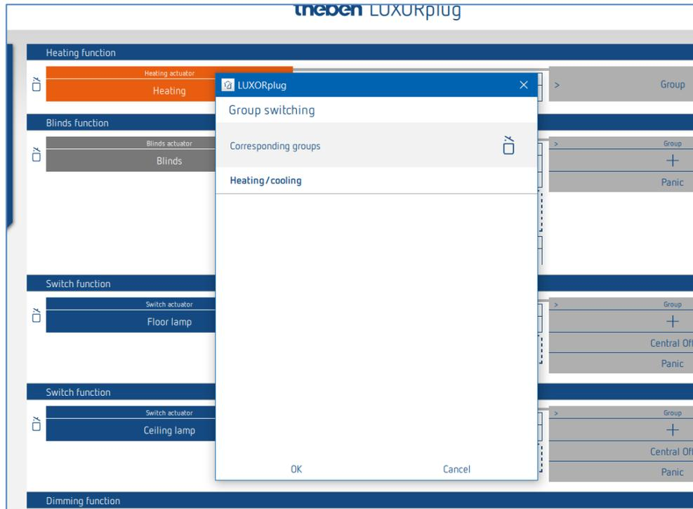
In control type "Heating and cooling", a "trigger", e.g. a channel of a button interface, can be drawn on the "Heating / cooling" group function, and the configuration type can be set.
