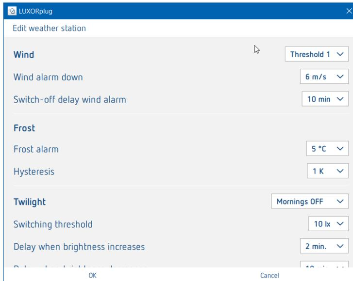
The "Frost" function prevents the automatic lowering of hangings when there is a risk of frost and allows the performance of a defined action in case of frost alarm. Participation and operation in case of frost alarm can be set for each blinds function individually in room view.
