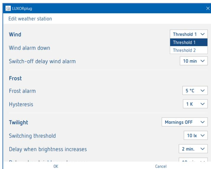
For each wind channel (threshold 1 and threshold 2), wind speed and switch-off delay can be set individually. The wind speed has to be set after consulting the technician or manufacturer of the hangings.
