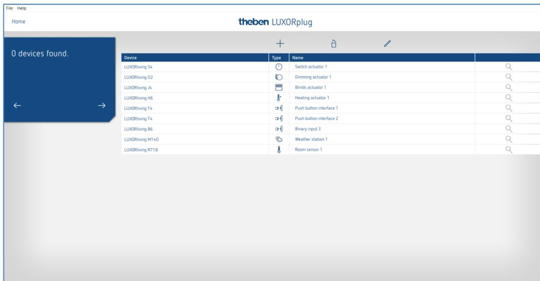
The arrangement of the devices in the left column (devices) can be adjusted by clicking, holding and moving.
