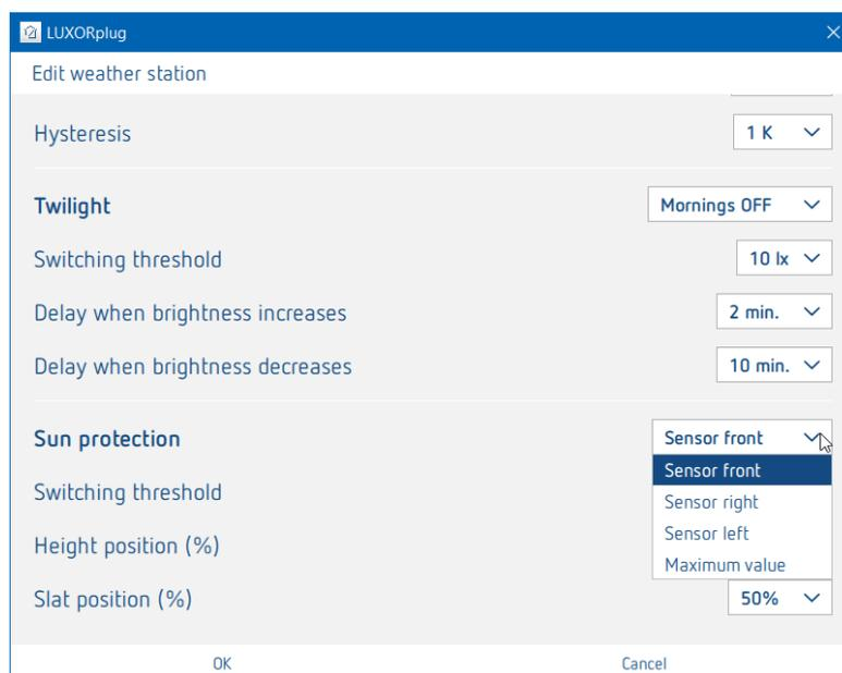
The "Sun protection" function includes four different functions. In room view, each of these functions can be assigned individually to the blinds functions.
