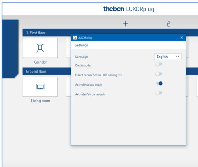
Debug mode can be activated by clicking five times on the free space. It is used for troubleshooting in the configuration.
