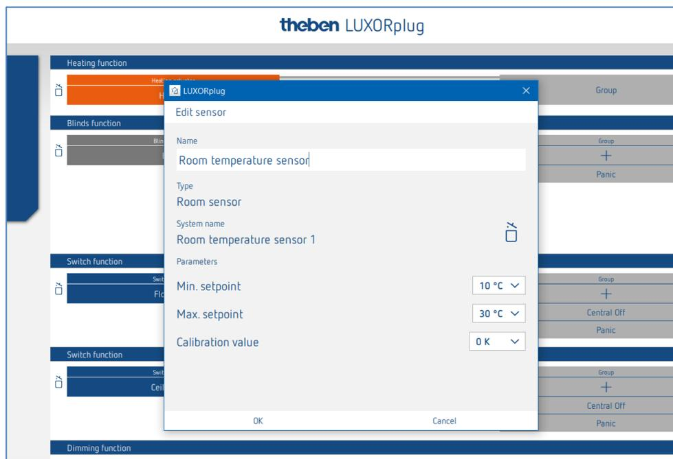
In the parameter window, the function can be named and various parameters can be set.
