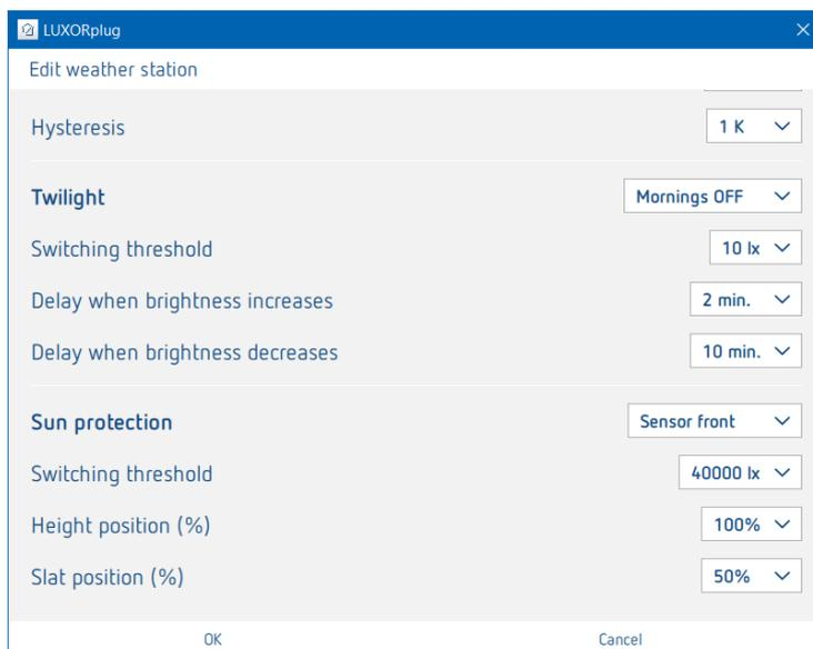
The "twilight" function includes four different dimming functions. In room view, each of these functions can be assigned individually to the switch, dimming, and blinds functions.
