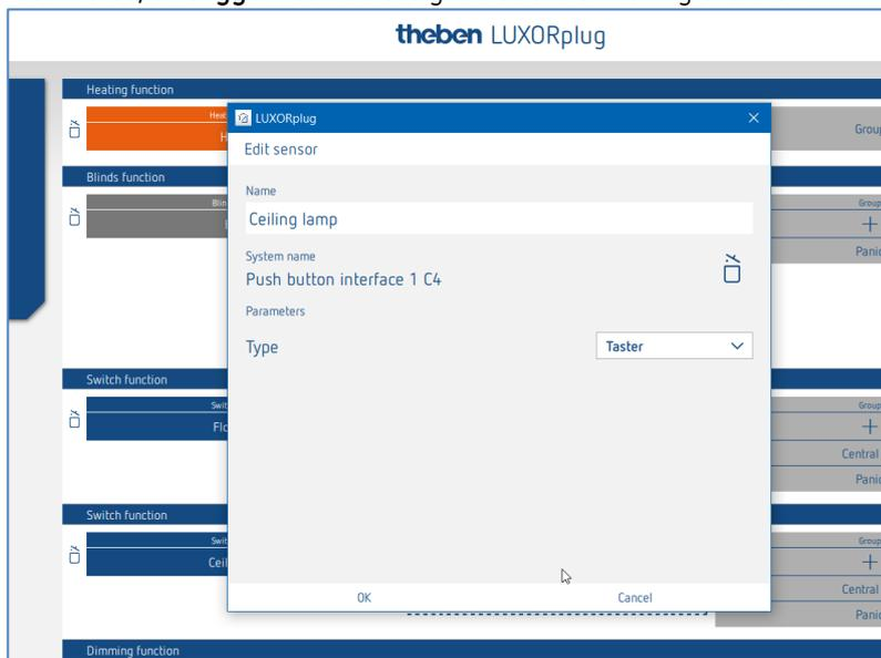
In the parameter window, the function can be named and various parameters can be set.
