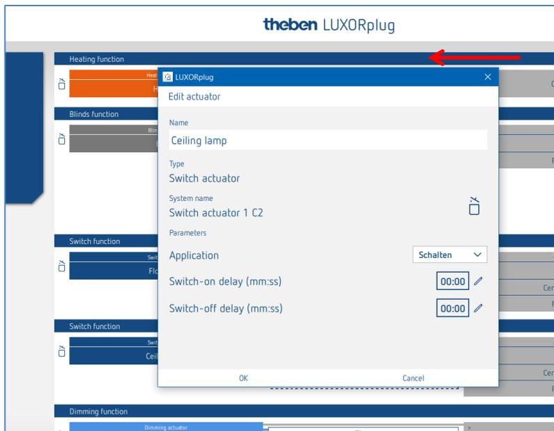
In the parameter window, the function can be named and various parameters can be set.
