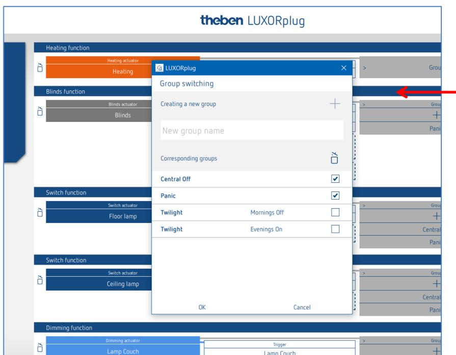
Here, the channel can be integrated into existing group functions, and own groups can be added. The thresholds for twilight functions can be set in the settings of the weather station.
