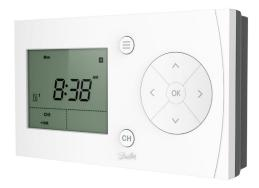
FP720 & TS710 heating timers provide flexible schedule setups to suit your lifestyle and ensure that heating is only called for during the normal home routine. The timers are used to switch your gas boiler either directly or via motorised zone valves and when used together with room thermostats can provide full heating and comfort control.
